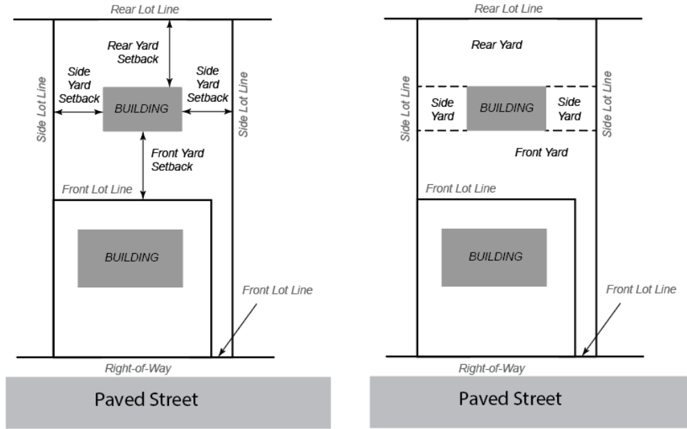
Figure 4-G: Typical lot lines and setback locations for a flag (panhandle) lot (left image) and typical yard locations (right image).
