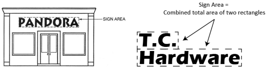
Figure 10-D: Illustration of sign area calculation for two differently shaped wall signs with individual letters.
